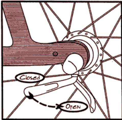
**Removing the wheel:** You'll have to either loosen the bolts or open the quick release. Note that quick releases aren't just bolts; most will have an "open" and "closed" side printed on the lever. You open quick releases by pulling them away from the bike, and close them by squeezing them against the frame.
