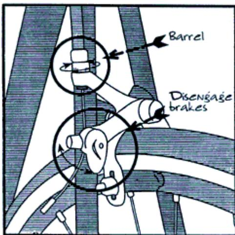
**Tightening your brakes:** Since brake pads wear and cables stretch, most brakes have a "barrel" adjuster at the end of the cable. This allows you to tighten the brake by lengthening the housing inside which the cable runs. Simply unscrew the barrel adjuster and then retighten the lock nut and you've got tight brakes for a bunch more miles.
